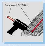
Application by means of a hot melt gun
